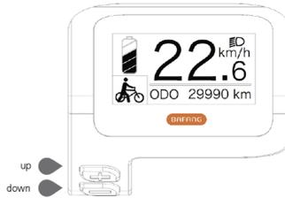
(b) Press and hold the Y switch again to run the motor in walk assist mode.
