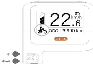
(c) Release the Y switch to stop the motor assist movement.
